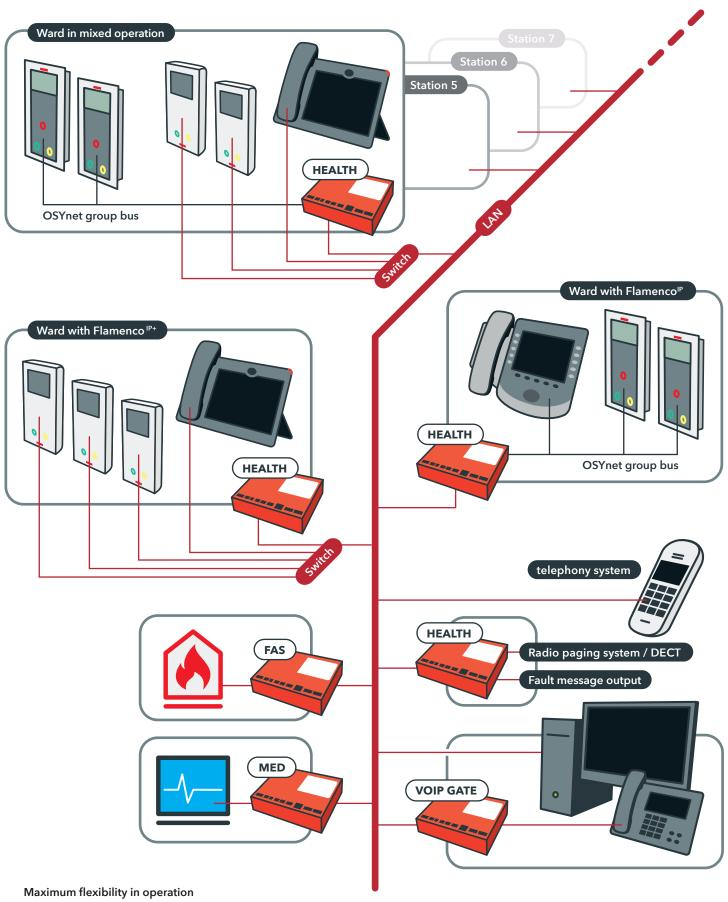
The IP-SystemManager allows wards to simultaneously use IP and BUS components and, thanks to various software system modules, enables the integration of PBX or fire alarm systems, for example.
